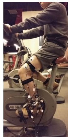
Figure 2: The data acquisition process of sEMG signals and joint angles signals during cycling exercises from one subject
